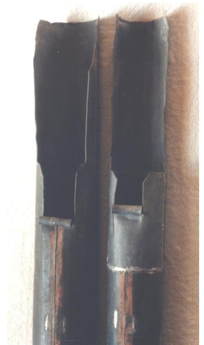
Lorentz lead pipes E and C pitch radically altered by Frobenius by cutting tuning coils (E with new piece of rolled lead inserted)
