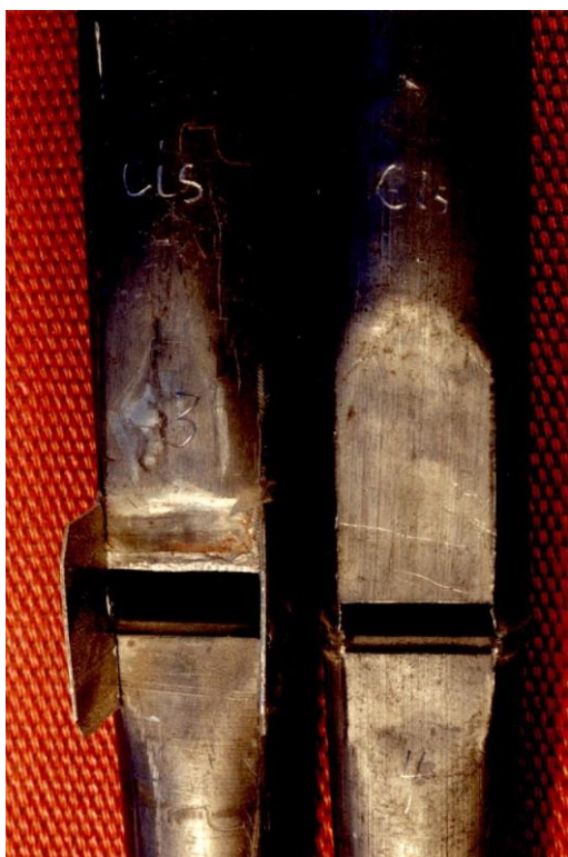
Malmö Petri organ: two 2' tenor c# pipes. Left: former Querpfeife (cut up later heavily remodeled, ears added). Right: Superoctava. Both pipes (of identical diameter) representing the same tradition as Lorentz inner pipes.
