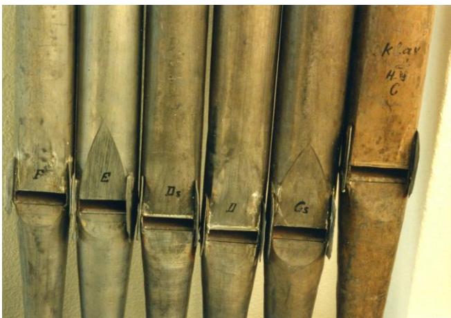
The present Octava 2' is a collage of older pipes. No. 2 from right may be the earlier bottom C in 'Chor-Thon' - the pipe far right is at present the bottom C pipe according to standard pitch - it is in reality the recycled former Lorentz Principal 4' bottom A pipe, of the standard make for pipes inside the case.
