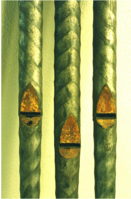
Embossed Brebosch dummy front pipes of pure tin (small holes of tin lepra mainly around lips)
