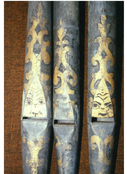
Front pipes from former Rückpositiv middle tower, now only on display. Left: the G-pipe body recut as 'Spitzflöte', on the F-languid (and foot). These pipes were never overpainted
