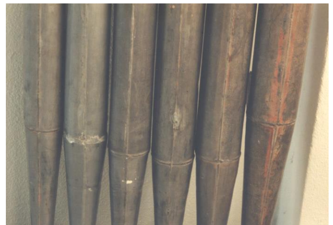
Rear view of the same pipes. The Lorentz former A pipe still displays the pipemaker's red size along the soldered seams which was never washed off (frequently also seen in such pipes made by Herman & Eijsenmenger).
